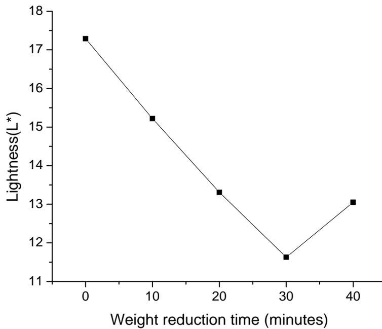
Fig.4 Variation of the lightness of the polypyrrole coated fabrics versus weight reduction time
