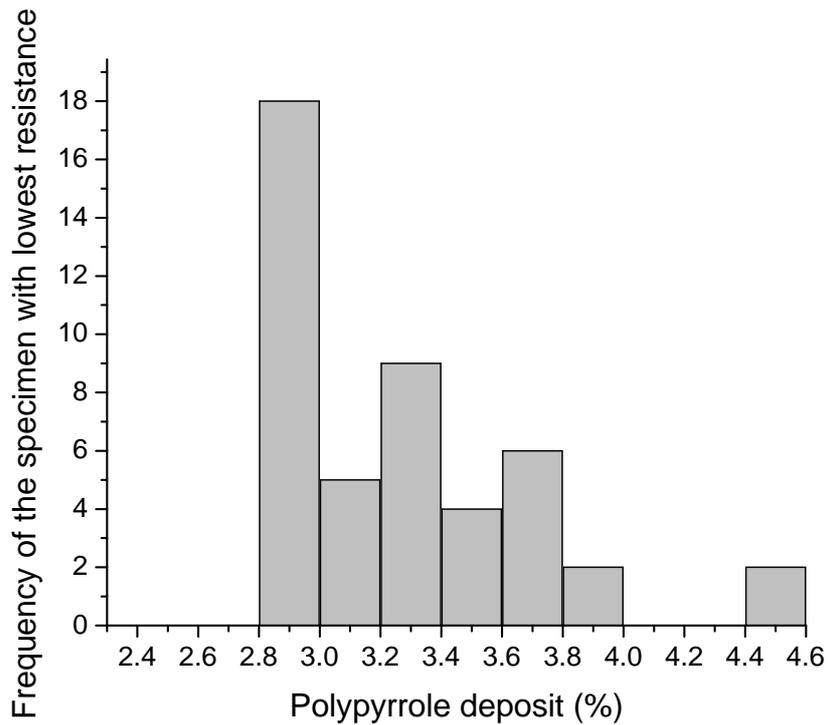
Fig.3 Histogram of the frequency of the weight reduced PET fabric specimen with lowest resistance versus polypyrrole take-up
