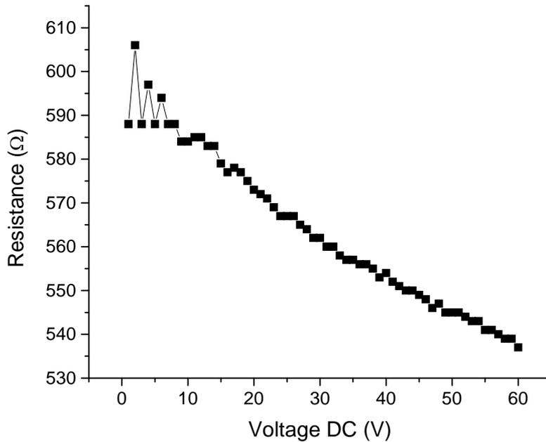
Fig.8 Variation of the resistance of polypyrrole coated weight reduced PET fabric versus voltage (Isotherm - Direct current) ( Weight reduction = 16.4%, Polypyrrole deposit = 3%)
