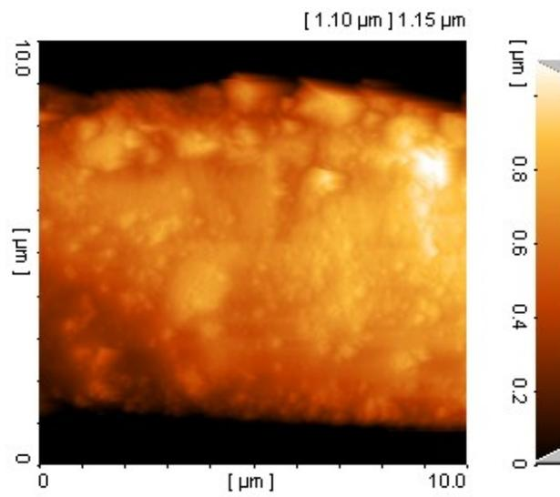
Fig.11 AFM image of polypyrrole coated PET fabric (weight reduction time 10 min.)
