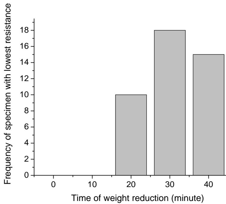
Fig.2 Histogram of the frequency of weight reduced PET fabric specimen with lowest resistance versus weight reduction time
