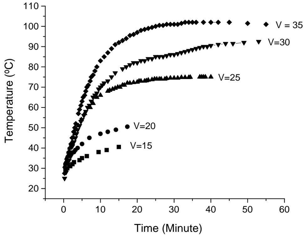
Fig.6 Variation of the temperature of polypyrrole coated weight reduced PET fabric with time (Weight reduction = 16.4%, Polypyrrole deposit = 3%)
