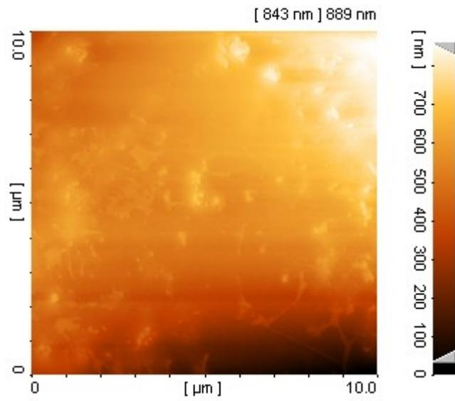
Fig.10 AFM image of polypyrrole coated PET fabric (untreated)
