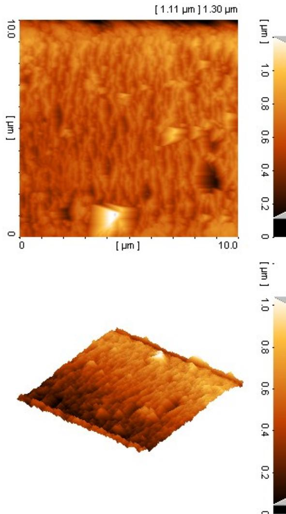
Fig.12 AFM image of polypyrrole coated PET fabric (weight reduction time 40 min.)
