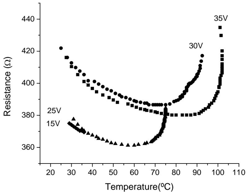
Fig.7 Variation of the resistance of a PPy coated weight reduced PET fabric with temperature (Weight reduction = 16.4%, Polypyrrole deposit = 3%)
