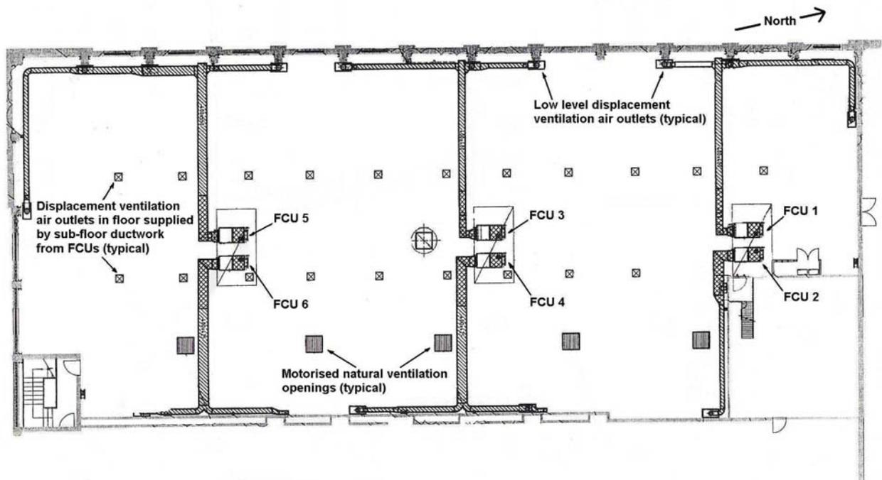
**Figure 2 Layout of the HVAC Scheme used in A+B Studio**
