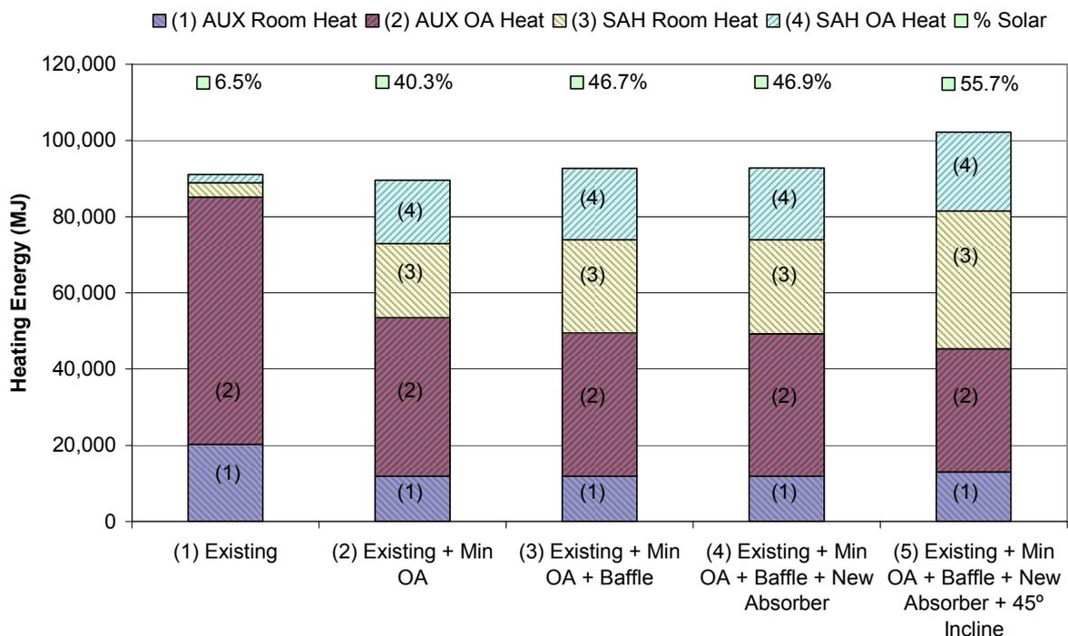
**Figure 7 Heat use for existing & modified SAH design & operation during March to August 2006**
