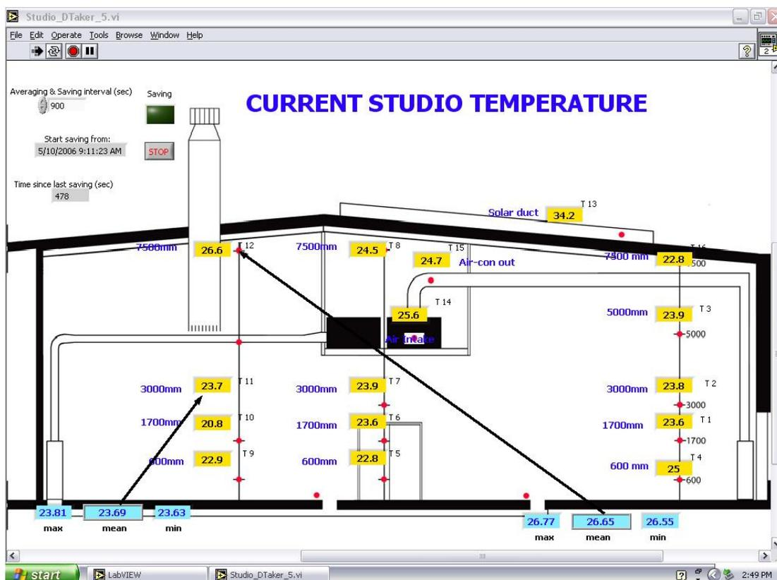
Figure 5 LabVIEW front panel display of thermistor readings in the A+B Studio
