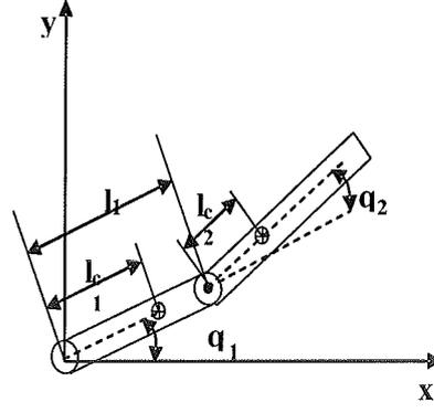
Fig. 1: Schematic of the Pendubot
