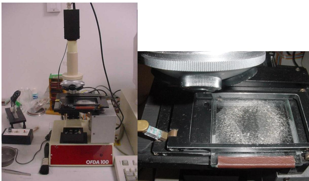
*Figure 3: The OFDA instrument (left) and an enlarged view of a slide of fibre snippets (right)*
