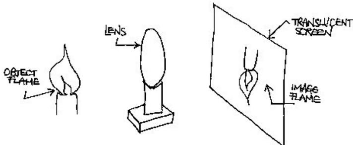
The image can be seen on both sides of the translucent screen. In comparing the image to the original flame the features are: \_\_\_\_\_
