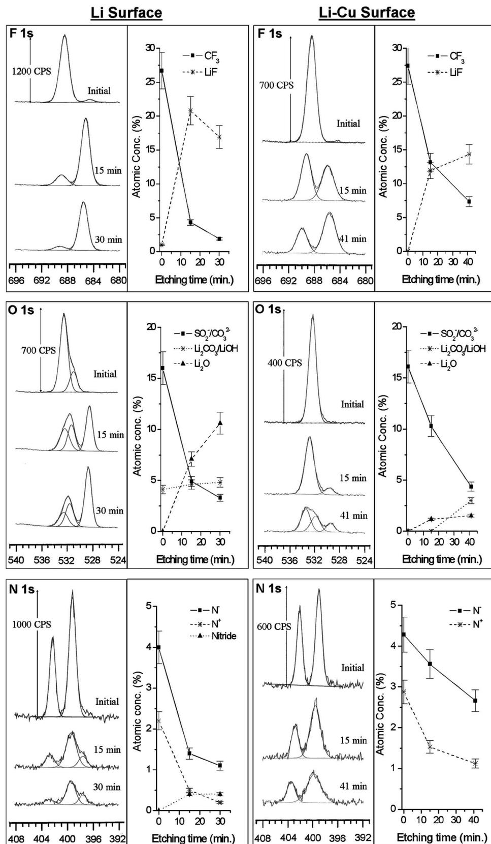
Figure 2. High-resolution F 1s, O 1s, and N 1s photoelectron spectra for the Li and Li-Cu surfaces before and after etching.
