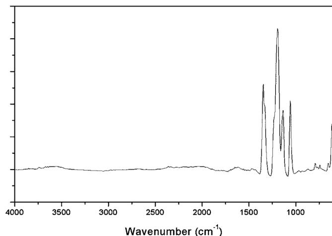
**Figure 6.** FTIR difference spectra obtained by sampling the surface of a separator taken from a cycled  $\text{Li}/0.5 \text{ mol kg}^{-1} \text{Li}(\text{Tf})_2\text{N-p}_{1.3}(\text{Tf})_2\text{N}/\text{Cu}$  cell.
