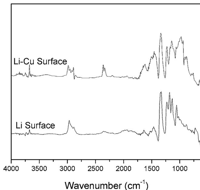
**Figure 5.** FTIR difference spectra obtained for the cycled Li-Cu surface, and the cycled Li surface.
