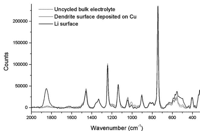
**Figure 7.** In situ Raman spectra acquired from a cycled optical cell containing  $0.5 \text{ mol kg}^{-1} \text{Li}(\text{Tf})_2\text{N-p}_{1.3}(\text{Tf})_2\text{N}$  showing a comparison of the bulk electrolyte, the Li surface, and the Li surface deposited on a copper substrate (dendrite surface).
