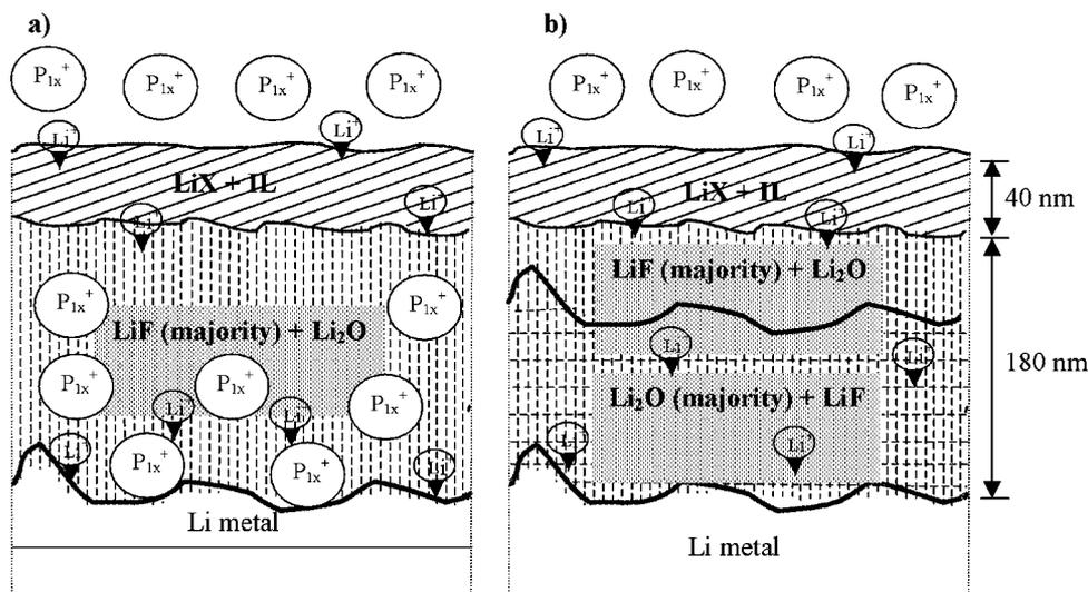
**Figure 12.** Simple models of the SEI structure on the Li (a) and the Li-Cu (b) surfaces.  $\text{LiX:X}$  can be  $\text{S}_2\text{O}_4$ , F,  $\text{SO}_3\text{CF}_3$ ,  $\text{NSO}_2\text{CF}_3$ ,  $\text{SO}_3$ ,  $\text{CO}_3$ , S, O, or OH.
