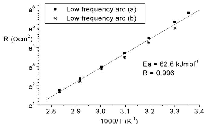
**Figure 10.** Arrhenius plot of the low-frequency arc resistance versus temperature for a cycled  $\text{Li}/0.5 \text{ mol kg}^{-1} \text{ Li}(\text{Tf})_2\text{N-p}_{1,3}(\text{Tf})_2\text{N}/\text{Li}$  cell: (a) temperature increasing, (b) temperature decreasing.
