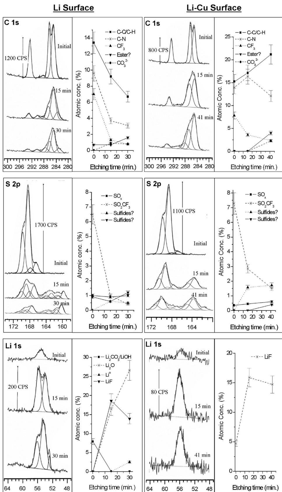
Figure 3. High-resolution C 1s, S 2p, and Li 1s photoelectron spectra for the Li and Li-Cu surfaces before and after etching.
