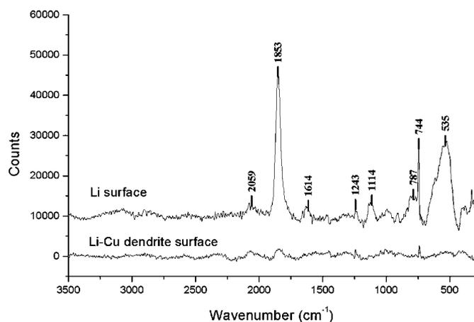
**Figure 8.** Raman difference spectra for the Li surface and the Li surface deposited on a copper substrate (dendrite surface) acquired from a cycled optical cell containing 0.5 mol kg<sup>-1</sup> Li(Tf)<sub>2</sub>N-p<sub>1,3</sub>(Tf)<sub>2</sub>N electrolyte.
