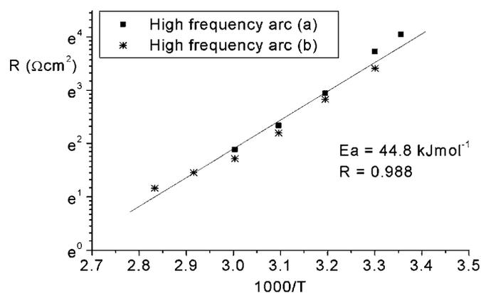
**Figure 11.** Arrhenius plot of the high-frequency arc resistance versus temperature for a cycled  $\text{Li}/0.5 \text{ mol kg}^{-1} \text{ Li}(\text{Tf})_2\text{N-p}_{1,3}(\text{Tf})_2\text{N}/\text{Li}$  cell: (a) temperature increasing, (b) temperature decreasing.
