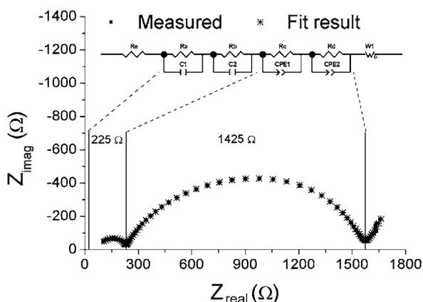
**Figure 9.** Example of a fitted impedance spectrum obtained from a cycled symmetrical lithium cell containing  $0.5 \text{ mol kg}^{-1} \text{ Li}(\text{Tf})_2\text{N-p}_{1,3}(\text{Tf})_2\text{N}$  electrolyte. The spectrum is fitted to a four-element layer model equivalent circuit; the error of the fit is shown.
