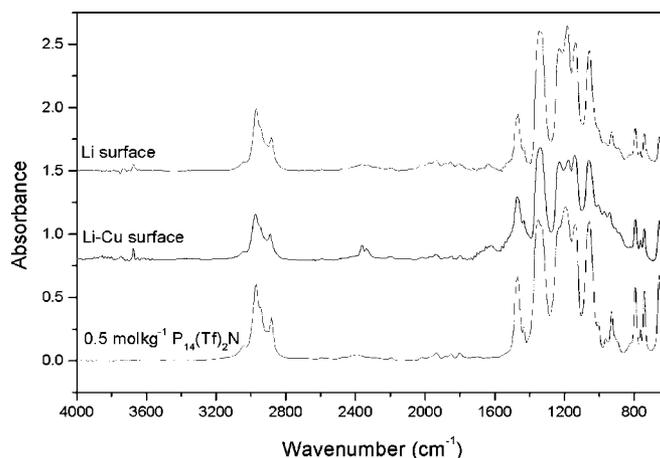
**Figure 4.** Comparative FTIR spectra for  $0.5 \text{ mol kg}^{-1} \text{Li}(\text{Tf})_2\text{N}-p_{1,4}(\text{Tf})_2\text{N}$  electrolyte (transmission mode), the cycled Li surface, and the cycled Li-Cu surface.
