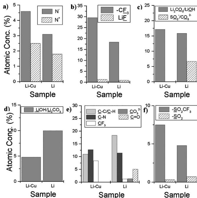
**Figure 1.** Atomic concentration (%) summary determined from the region spectra for the Li and Li-Cu surface (estimated error  $\pm 10\%$ ): (a) N 1s region, (b) F 1s region, (c) O 1s region, (d) Li 1s region, (e) C 1s region, (f) S 2p region.
