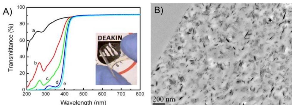
**Figure 5.** A) UV-vis spectra of (a) EVOH matrix and HMBS@LDH-EVOH nanocomposite films with HMBS@LDH loadings of (b) 2, (c) 5, (d) 10 and (e) 15 wt%, respectively. The inset shows a transparent and flexible film. B) TEM image of HMBS@LDH-EVOH nanocomposite film (15 wt% HMBS@LDH).
