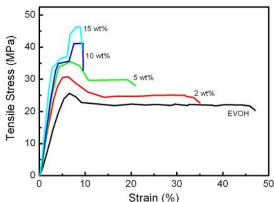
**Figure 6.** Stress-strain curves of pure EVOH and HMBS@LDH-EVOH nanocomposite films.
