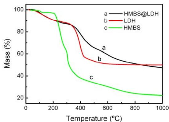
**Figure 4.** TGA curves of HMBS, LDH nanocrystals, and HMBS@LDH nanocrystals.
