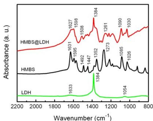
**Figure 3.** FTIR spectra of LDH, HMBS, and HMBS@LDH.
