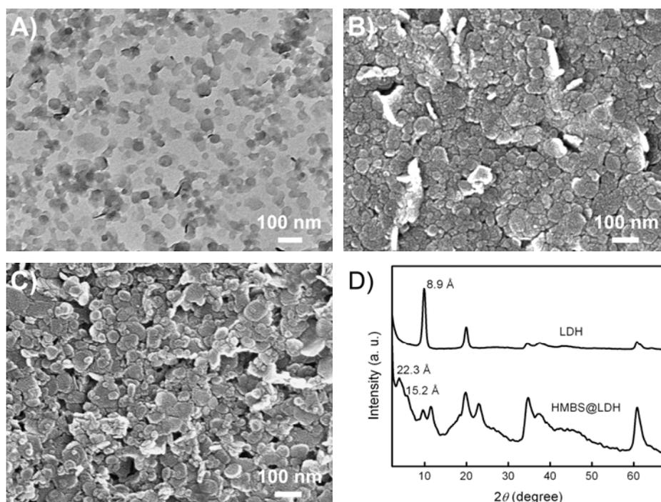
**Figure 1.** A) TEM and B) SEM images of the as-prepared LDH nanocrystals. C) SEM image of HMBS@LDH nanocrystals. D) XRD patterns of LDH and HMBS@LDH nanocrystals.
