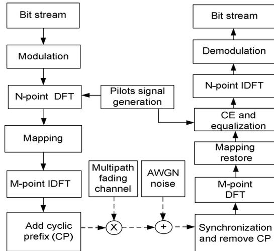
Fig. 2. LTE SC-FDMA transceiver system model.
