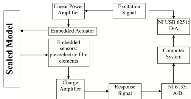
Figure 3: Guided wave test system
