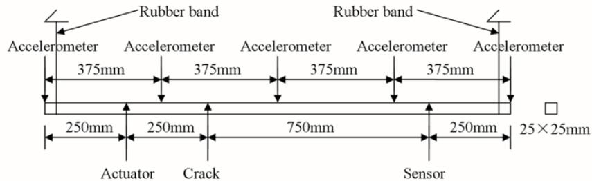
Figure 1: The specimen of steel beam
