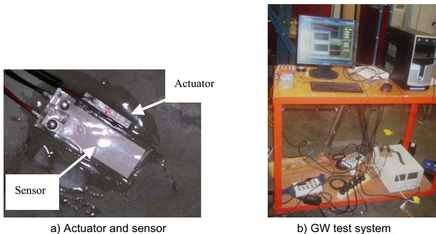
Figure 4: Photos of guided wave test system
