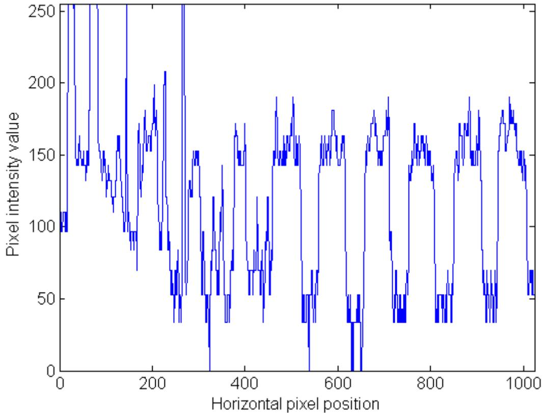
**Fig. 4.** A typical horizontal image data cross section from a ‘bad’ sample.
