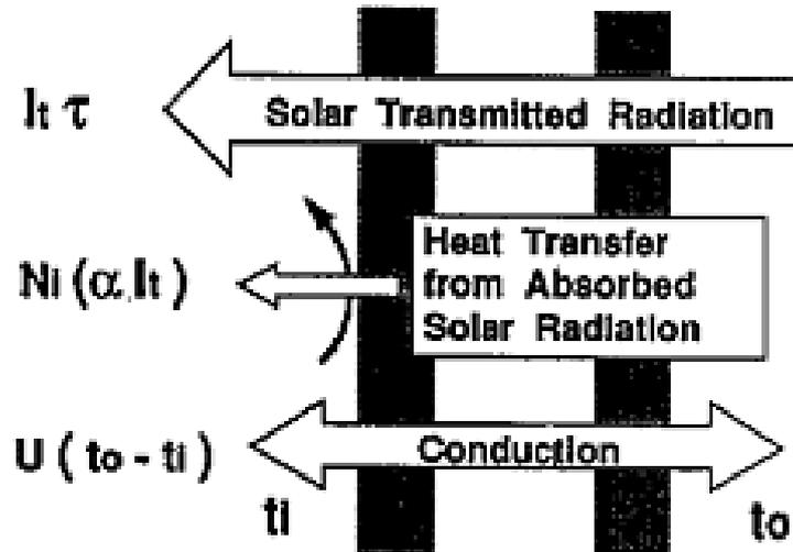
Figure 3: Heat transfer in a double glazed window (Luther, 1995)
