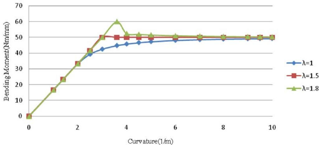
**FIGURE 14.** Theoretical moment–curvature diagram in bending aged materials without tension.
