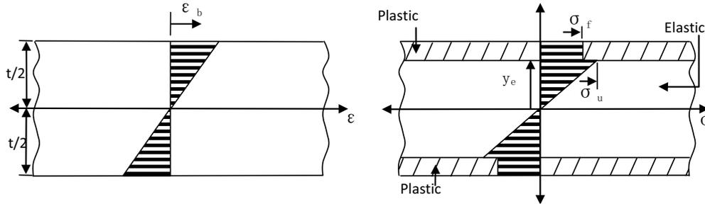
FIGURE 13. Assumed strain and stress distribution in bending of aged sheet.
