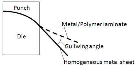
**FIGURE 7.** Schematic of a homogeneous metal strip and a metal/polymer/metal laminated sheet clamped between dies of circular profile showing the difference in the shape of the free standing strip (Gullwing defect).
