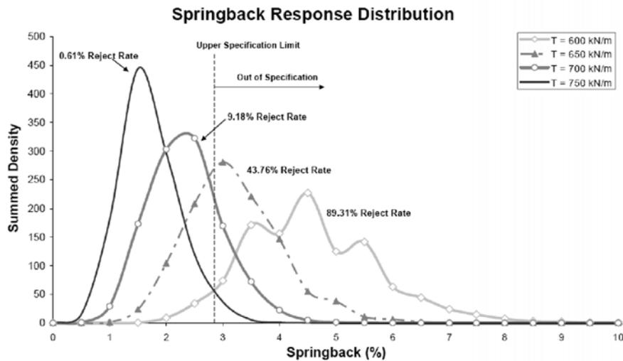
FIGURE 4. Springback distributions for a range of sidewall tensions and reject rate given an upper specification limit.
