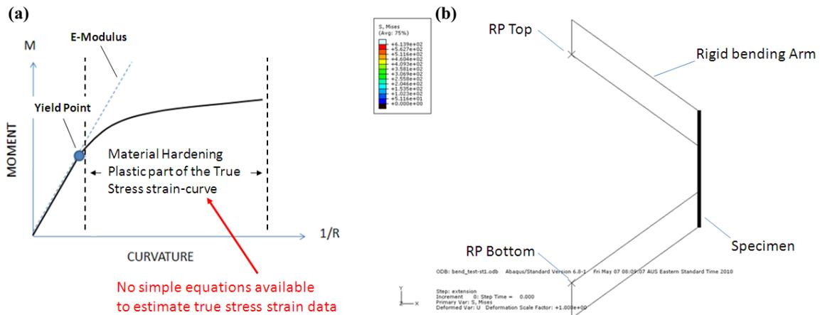
FIGURE 10. a) Moment curvature diagram determined in the pure bending test. b) Numerical model of the bending test.
