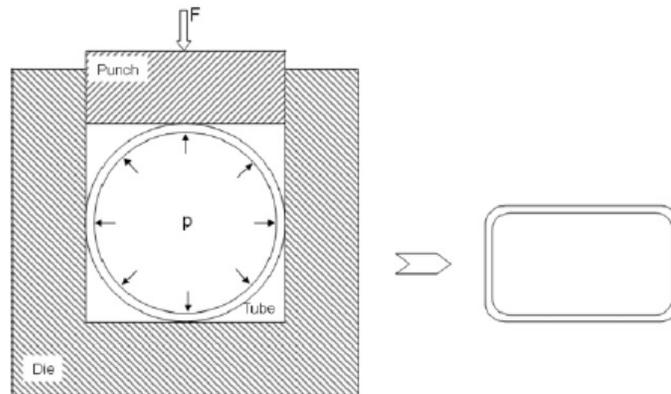
**FIGURE 8.** Schematic of low pressure hydroforming and the part shape analysed.
