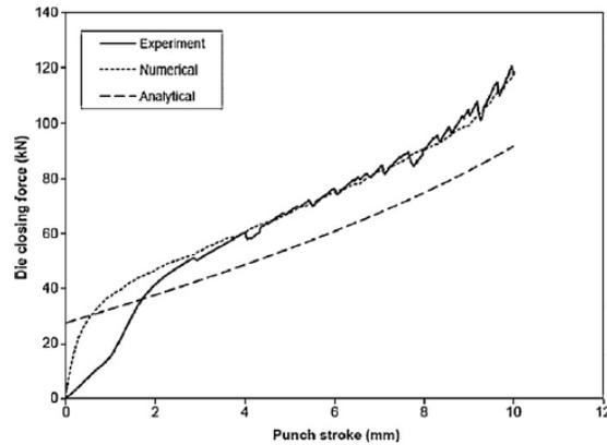
FIGURE 9. Die closing forces for the forming of a pressurized tube (10 MPa) at 10 mm die displacement.
