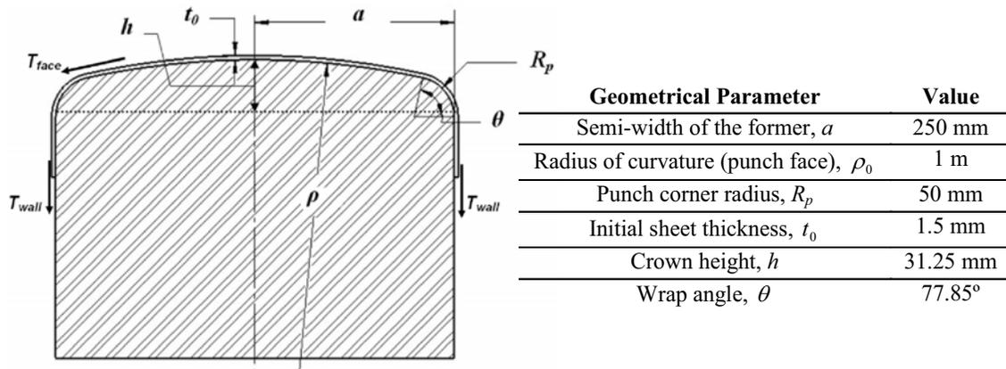
FIGURE 3. Two-dimensional stretch forming operation.
