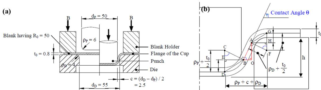
**FIGURE 1.** (a) Schematic diagram of the deep drawing of a cylindrical cup (dimensions in millimeters) and (b) Geometry of deep-drawn cup for determination of the contact angle  $\theta$ .
