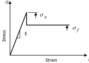
FIGURE 12. Assumed stress strain relation in aged sheet.
