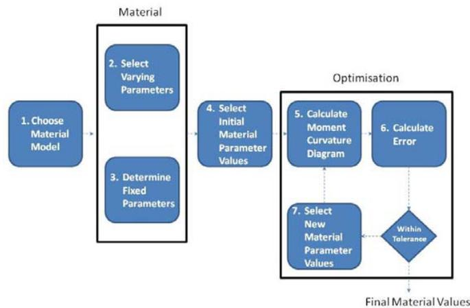
FIGURE 11. Schematic of the inverse model used showing the seven main steps.
