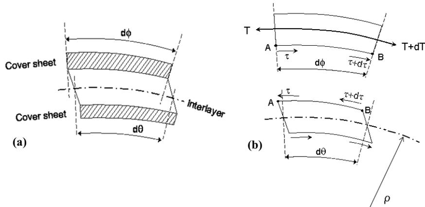
FIGURE 5. a) An element of the laminate material bent at a constant radius of curvature. b) Force equilibrium diagram of both the cover sheet and the interlayer.
