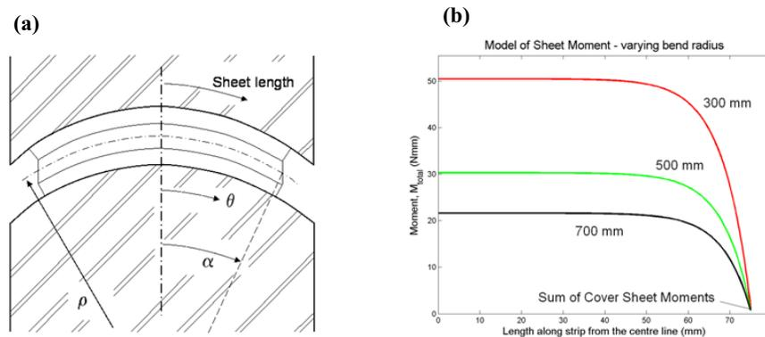
FIGURE 6. a) Bending of the metal/polymer laminate material to a constant radius of  $\rho$  for a frictionless clamped die. b) The moment diagram of the metal/polymer laminate bent to a circular arc for different values of the bend radius.
