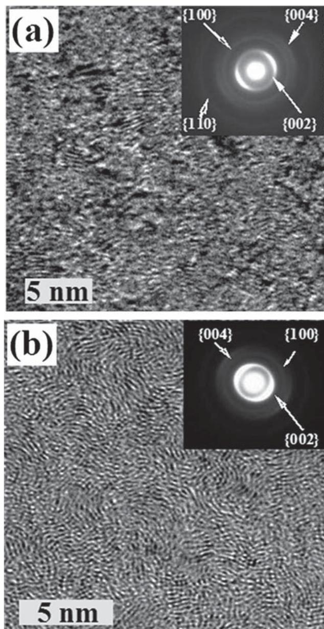
**Fig. 3** TEM images of oriented carbon films prepared at (a) low and (b) high temperatures. The inset in each image is an electron diffraction pattern indexed to graphite.
