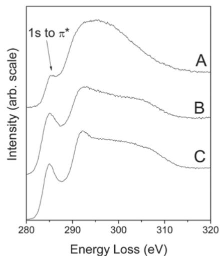
**Fig. 4** Carbon K edges from oriented carbon films grown at (A) low temperature (B) high temperature and (C) a bulk glassy carbon sample.
