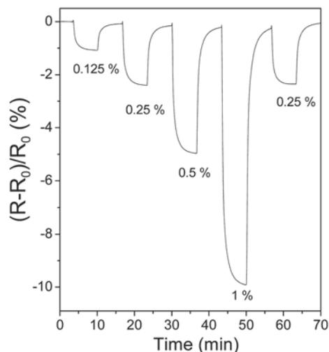
**Fig. 6** The normalized change in resistance upon exposure to the indicated concentrations of hydrogen in synthetic air measured from the type B sensor at 120 °C with a central Pt pad and made using the low temperature carbon films. Note that this measurement was made in two-probe configuration using a single contact at each end of the sensor.
