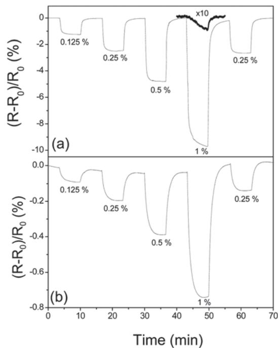
**Fig. 5** The normalized change in resistance during the exposure to the indicated concentrations of hydrogen in synthetic air in type A sensors at 120 °C made from (a) low and (b) high temperature carbon films. Also shown in (a) is the response of this sensor at room temperature (thick solid line) to 1% hydrogen magnified by a factor of 10.
