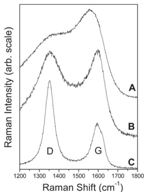
**Fig. 2** The Raman spectrum of the carbon films prepared on quartz at temperatures of (A)  $100\text{ °C}$  and (B)  $600\text{ °C}$ . Included is (C) the Raman spectrum from a bulk sample of glassy carbon heat treated to  $3000\text{ °C}$  showing the characteristic D and G peaks produced by disordered graphitic materials.
