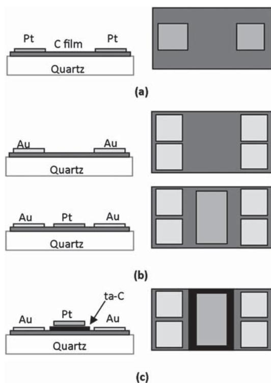
**Fig. 1** Cross-sectional (left) and plan view (right) representations of the (a) 'type A', (b) 'type B' and (c) 'type C' conductometric hydrogen gas sensors incorporating oriented carbon films. Note that the type B sensor was fabricated with and without a central catalytic Pt pad and the Pt pad in the type C sensor is electrically isolated from the oriented carbon beneath using a tetrahedral amorphous carbon layer.
