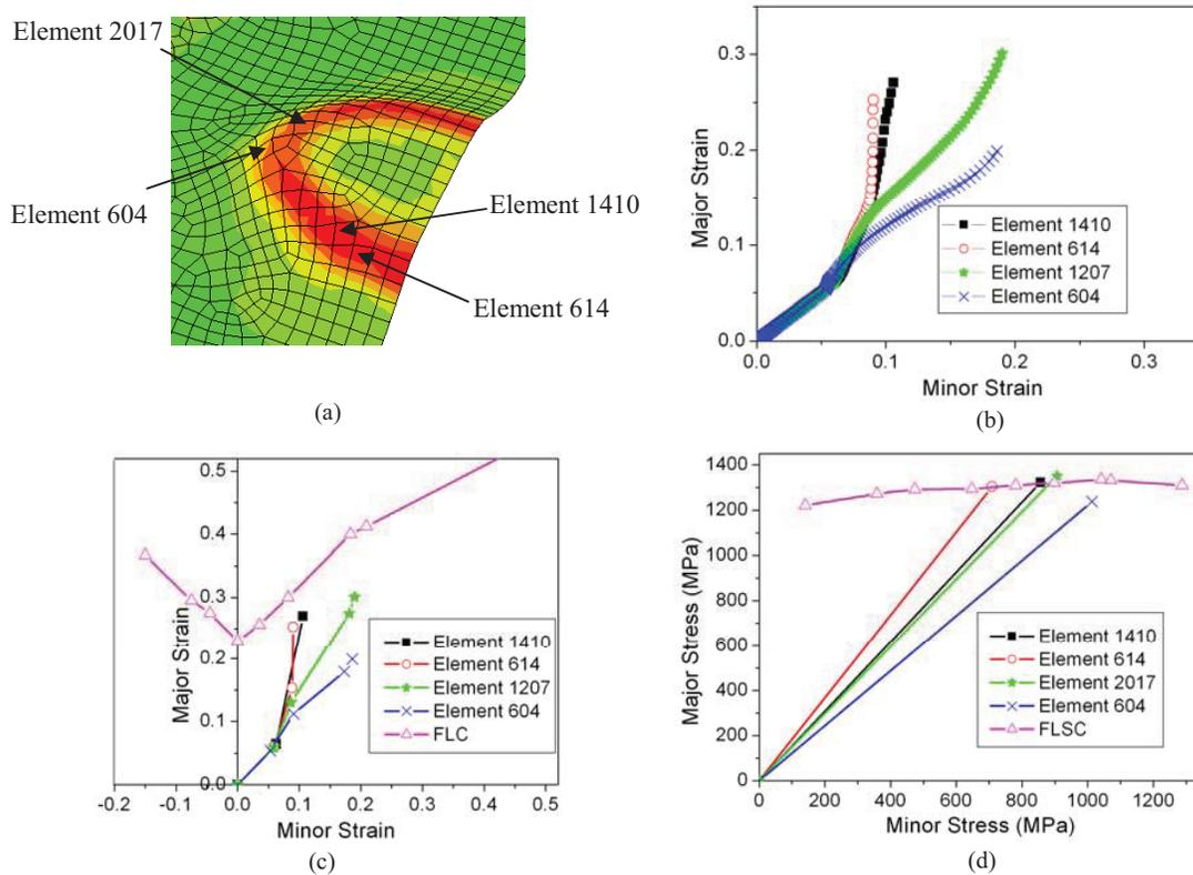
**FIGURE 5.** Results with Different Forming Limit Diagram
