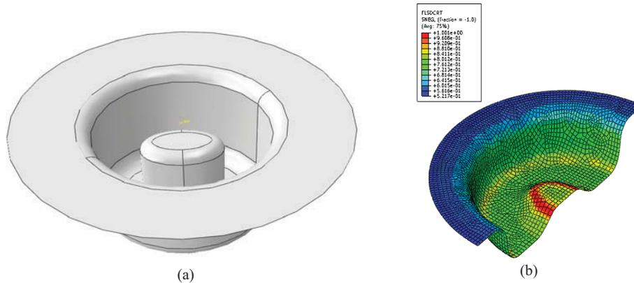
**FIGURE 4.** Die Shape and Simulation Result for DP780
