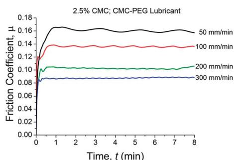
Fig. 6 Effect of shearing velocity on the friction response of a CFN disk modified with a 2.5% CMC solution against a stainless steel 'pin' (*i.e.* in a migrating contact position geometry) using a 1% wt CMC-PEG in PBS lubricant solution. All the measurements were performed using a static load of 1 N (approximate pressure at the center of contact  $\approx$  0.3 MPa).
