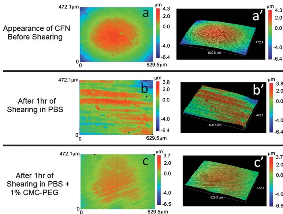
Fig. 5 Optical profilometry images showing the 2d (a–c) and 3d (a'–c') surface topography of CFN pins modified with a 2.5% CMC solution measured before shearing (a and a'), after 1 h of shearing in PBS lubricant (b and b'), and after 1 h of shearing in PBS containing 1% wt CMC–PEG boundary lubricant. Shearing was performed at a shear rate of  $50 \text{ mm min}^{-1}$  against a stainless steel disk under a constant load of 3 N.
