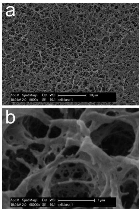
Fig. 1 SEM micrographs showing the CFN microstructure at (a) low and (b) high magnification. Samples were prepared by freeze drying in order to preserve the 'swollen' structure of the CNF and were coated with a roughly 30 nm thick conductive gold film for imaging.
