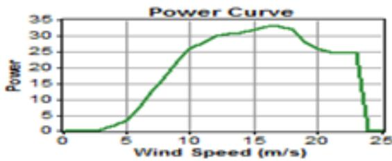
Figure 8: Wind turbine power curve
