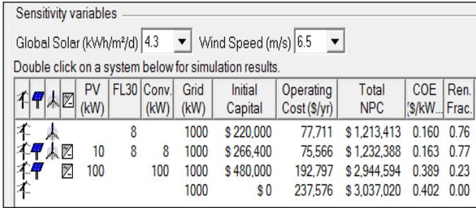
Figure 12 : sensitive analysis (with maximum wind speed sensitive value)
