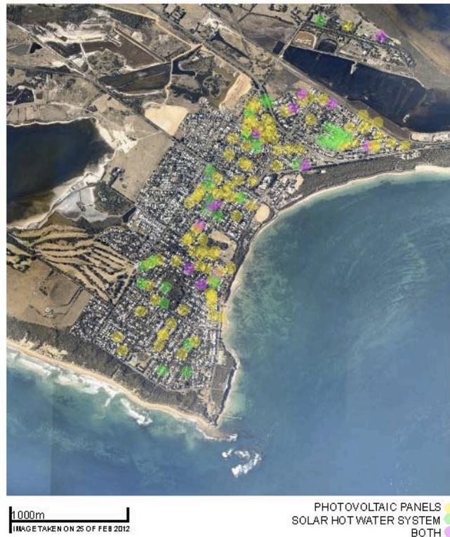
**Figure 1: Distribution of solar PV and hot water systems in Point Lonsdale on the 25/2/2012**
