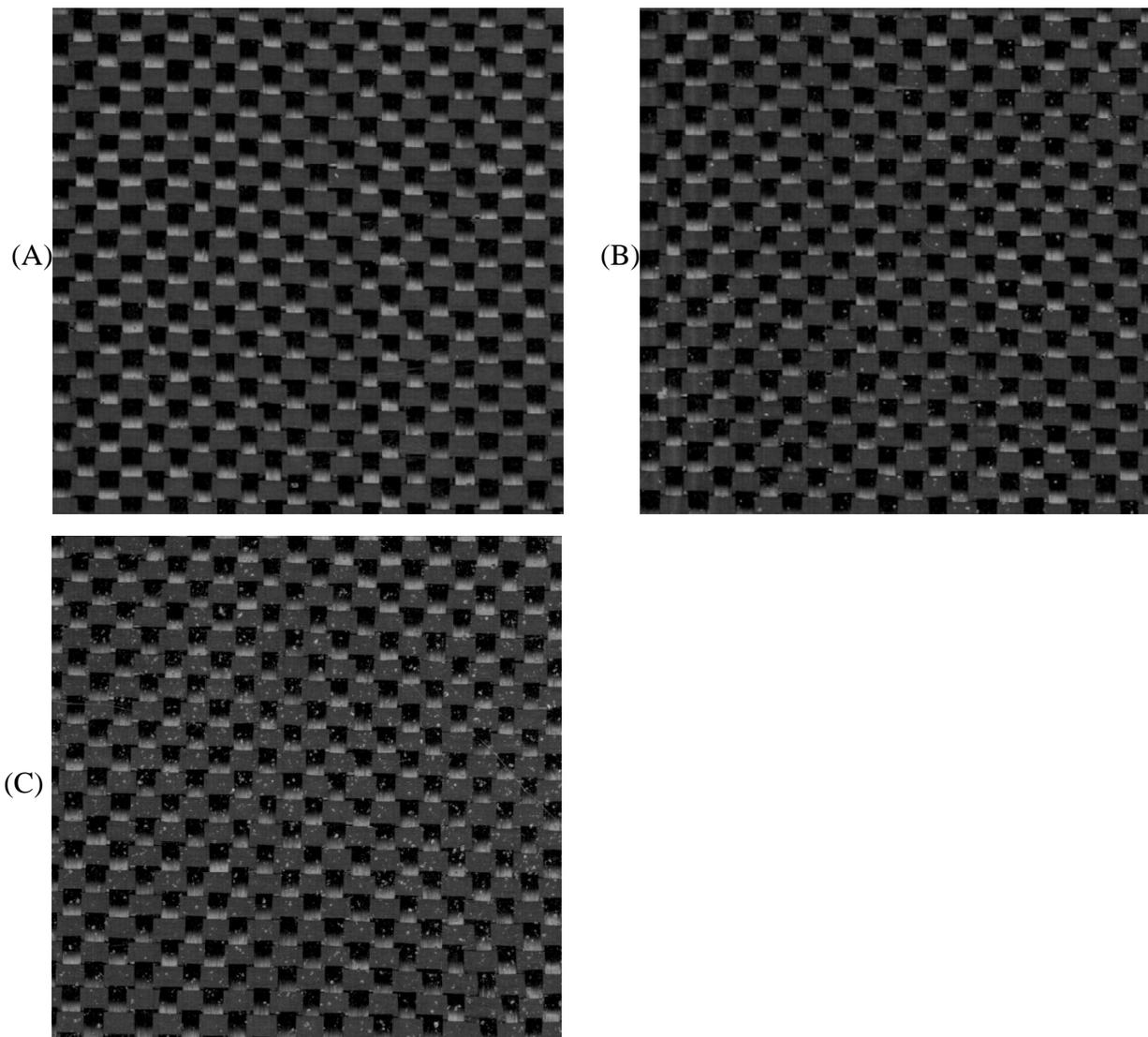
Fig. 1 Typical sample test images for (A) grade 1; (B) grade 2; and (C) grade 3 surface finish
