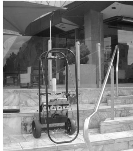
Figure 2: The mobile laboratory comfort carts used in measurement.
