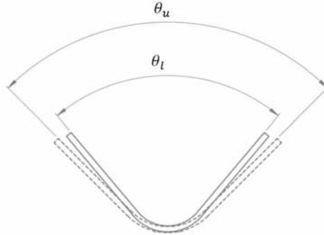
**Figure 6** Representative diagram for the multi-step V-die bending test
