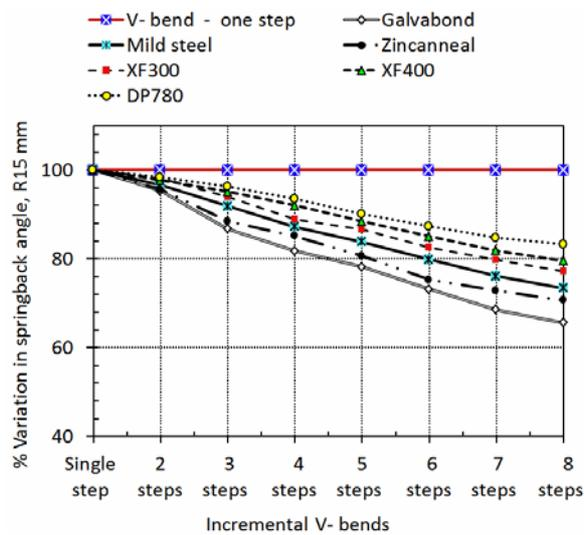
**Figure 12** Variation (%) in springback with incremental V-bending for R5 (see online version for colours)
