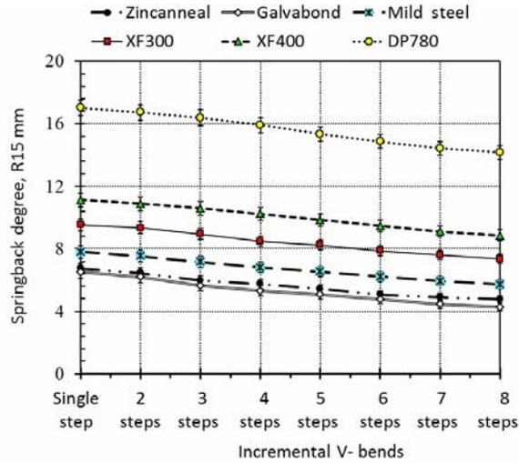
**Figure 9** Change of springback with incremental V-bending for R5 (see online version for colours)
