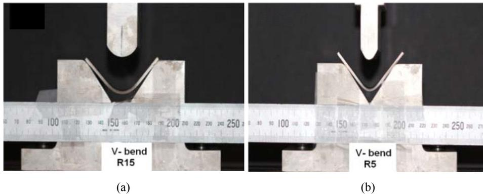
The springback was calculated using equation (1) as shown in Figure 5.
