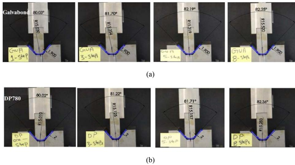
**Figure 11** Variation (%) in springback with incremental V-bending for R15 (see online version for colours)
