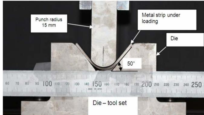
The springback was determined using an optical method; for this photograph was taken under loading (Figure 3) and after release (Figure 4). The angles under load,  $\theta_l$ , and after release,  $\theta_u$  were, measured using the CAD software package ‘SOLIDWORKS’.
