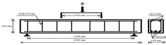
Figure 1: Beam cross- section.
