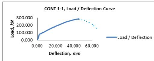
Figure 8: Load deflection Curve of the Control slab.
