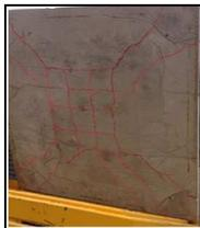
Figure 7: cracking pattern for control slab.
