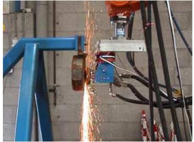
**Figure 5:** Grinding with IRB6400 at Kranendonk, the Netherlands, using a compliant grinding tool developed at KU Leuven, Belgium, together with force feedback control. The video can be found at [www.robot.lth.se](http://www.robot.lth.se).
