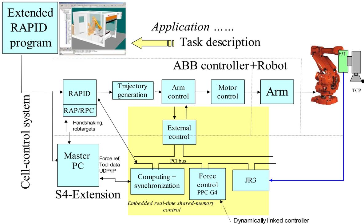
**Figure 2:** Extension of industrial robot controller with sensor interface and support for external computations and synchronization, using a Motorola PPC-G4 PrPMC-800 processor board mounted on a Alpha-Data PMC-to-PCI carrier board with a local PCI bus.
