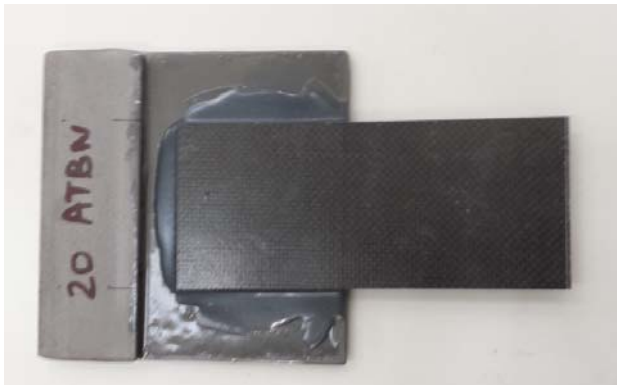
Figure 1. CFRP sheet bonded to the Steel plate
