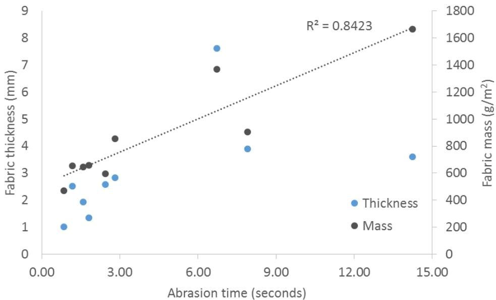
Fig. 3: fabric mass per unit area and fabric thickness with respect to abrasion time
