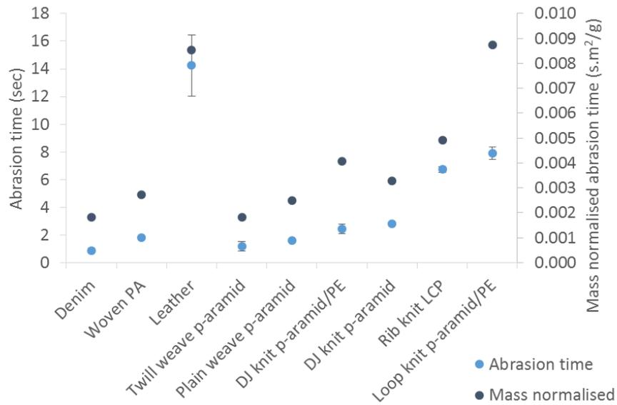
Fig. 2: abrasion resistance results of each fabric structure
