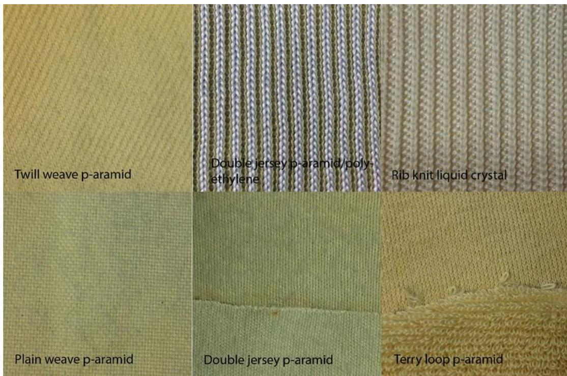
Fig. 1: protective layer fabric structure and fibre type
