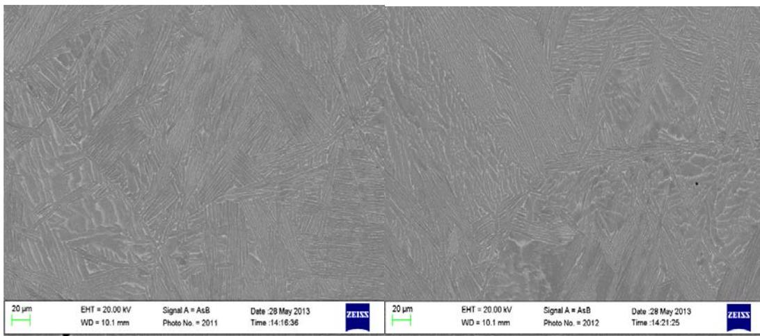
**Figure 6: SEM microstructure of machined Ti-6Al-4V alloy**
