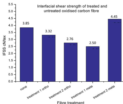
Fig. 11 Interfacial shear strength of treated and untreated samples. From left to right: control (oxidised and unsized fibre); fibres functionalised with **14** treatment 1 only, fibres functionalised with **14** treatment 2, fibres functionalised with **16** treatment 1 only, and fibres functionalised with **16** treatment 2.
