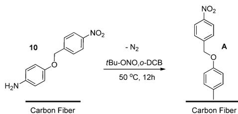
**Scheme 2** Surface functionalisation of carbon fibre with aniline **10**.
