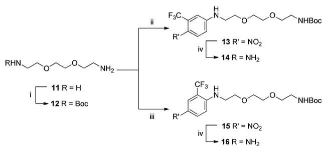
Scheme 3 Conditions: (i)  $\text{Boc}_2\text{O}$ ,  $\text{CH}_2\text{Cl}_2$ , 16 h; (ii) 5-fluoro-2-nitrobenzotrifluoride DMF,  $100^\circ\text{C}$ , 80 min; (iii) 2-fluoro-5-benzotrifluoride, DMF,  $100^\circ\text{C}$ , 80 min; (iv)  $\text{H}_2$ , Pd/C (10% w/w), MeOH, 16 h.
