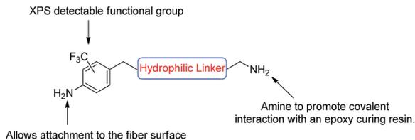
Fig. 3 Schematic of an ideal compound for attachment to the carbon fibre surface.
