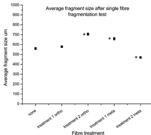
Fig. 10 Average fragment size from SFFT, from left to right: control (oxidised and unsized fibre); fibres functionalised with **14** treatment 1 only, fibres functionalised with **14** treatment 2, fibres functionalised with **16** treatment 1 only, and fibres functionalised with **16** treatment 2. Statistically significant results denoted by \*.
