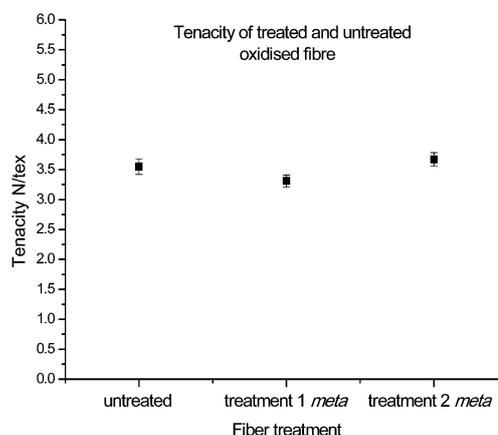
Fig. 5 Tenacity of single fibres having undergone functionalisation with **16**.
