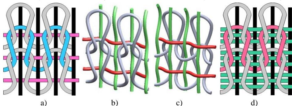
Fig. 1: The designed structures. a) basic structure; b) & c) 3D sketches of basic structure; d) improved structure
