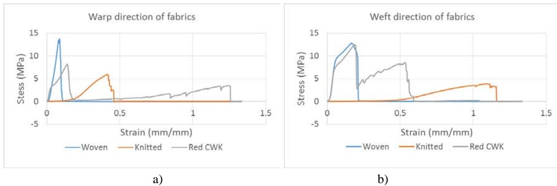
Fig. 4: Stress-strain curves of woven, knitted and CWK fabrics. a) warp direction; b) weft direction
