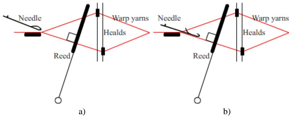
Fig. 2: The process of fabrication. a) needles at the back position; b) needles at the forward.
