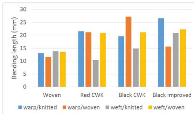
Fig. 6: Bending length of four fabrics
