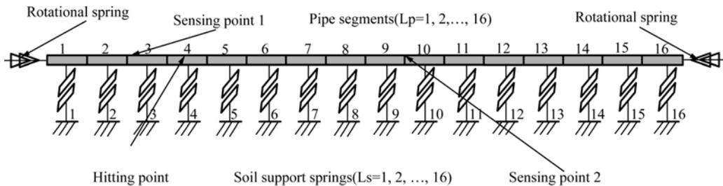
Figure 2. Simplified pipe-soil interaction finite element model
