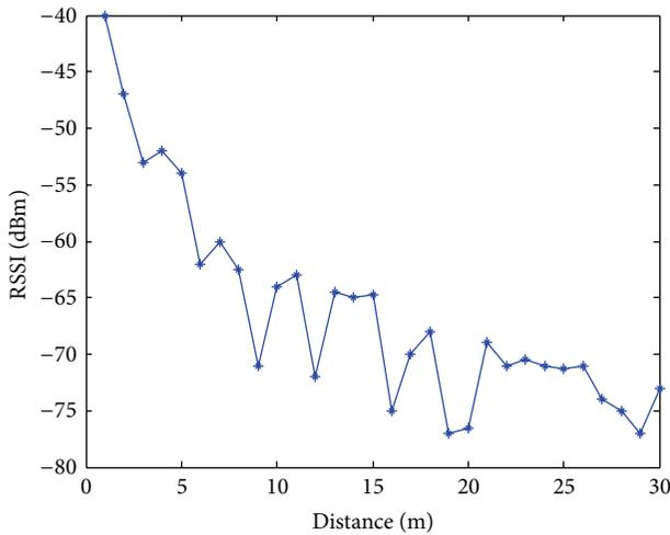
FIGURE 2: The relationship between RSSI attenuation value and distance.
