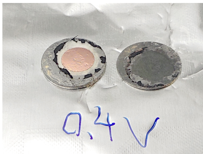
Figure S15. The photo of the components after charging to 0.4 V.
