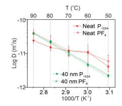
**Fig. 7** Comparison of the diffusion coefficients of the extrapolated diffusion coefficient of neat OIPC  $D_0$  to the 40 nm sample. The latter was obtained by a number averaging of the  $D_t$  values with different diffusion times.
