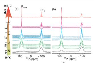
**Fig. 3** Stack plots of the variable temperature static <sup>31</sup>P NMR spectra of (a) neat OIPC and (b) the 40 nm sample, with separate peaks for cation and anion. The temperature was increased from 10 to 160 °C with a step of 10 °C. The solid transition temperatures are indicated on the arrow at left-side, and spectra of each solid phase are grouped and coded with a different color.
