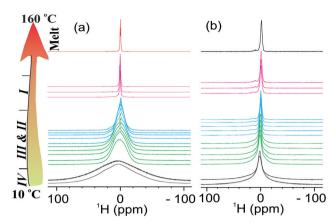
Fig. 4 Stack plots of the variable temperature static <sup>1</sup>H NMR spectra of cation in (a) neat OIPC and (b) 40 nm sample. The temperature was increased from 10 to 160  $^{\circ}$ C with a step of 10  $^{\circ}$ C.
