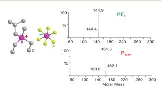
Fig. 1 Molecular structure and mass spectroscopy of the OIPC [P<sub>122i4</sub>][PF<sub>6</sub>].
