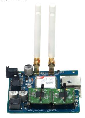
FIGURE 8. Radxa Board with Custom Built Hat Board
