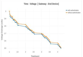
FIGURE 10. Time to Voltage Drain with and without the Authentication Code in Gateway-Edge Node Setup
