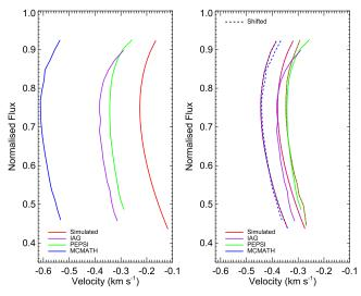
**Figure 4.** Left: average line bisector from the disk-integrated model observations (shown in red), alongside those from empirical data taken with the McMath (blue), IAG (purple), and PEPSI (green) instruments. Right: same, but model observations are convolved with IPs, and shifted for shape comparison; red-blue, red-purple, and red-green lines correspond to the McMath, IAG, and PEPSI instruments, respectively. The McMath data are also shifted (dashed blue).
