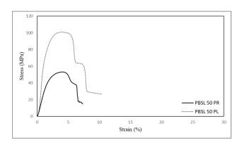
(a) Stress-strain curves for 50 mm specimens
