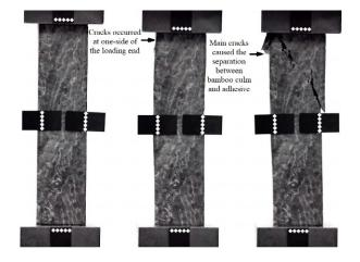
(c) Failure characteristics of PR specimens
