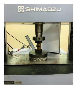
Fig. 2. Test set-up used for compression
