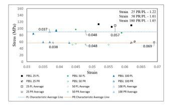
Fig. 8. Strain analysis for the tested PBSL specimens
