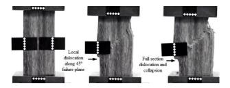
(b) Failure procedures of PL specimens
