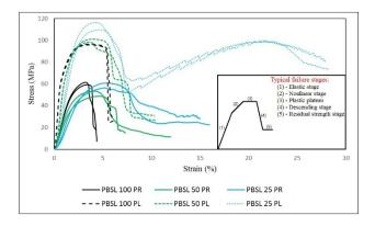
Fig. 6. Stress-strain behaviours of PBSL under compression tests
