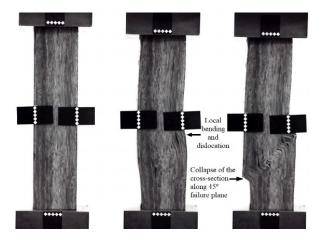
(b) Failure characteristics of PL specimens
