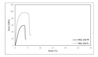
(a) Stress-strain curves for 100 mm specimens
