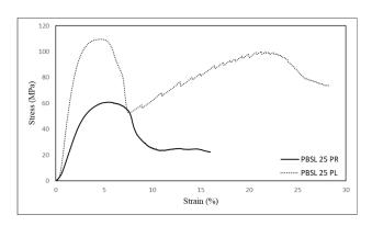
(a) Stress-strain curves for 25 mm specimens
