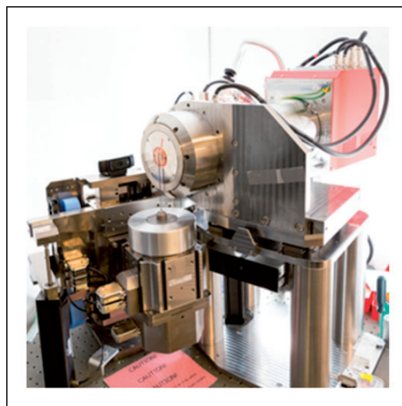
Figure 3. Experimental arrangement of the helical type micro computerized tomography scanner.
