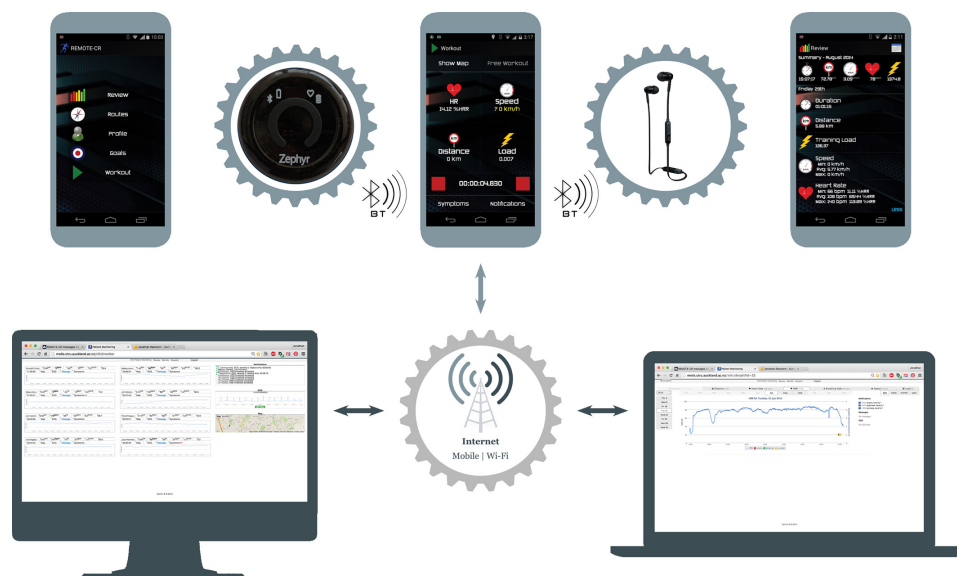
Figure 1 Remotely monitored exercise-based cardiac telerehabilitation platform schematic.
