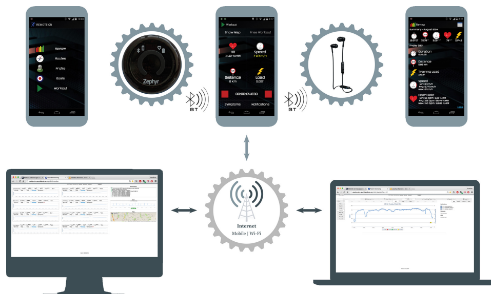
Figure 1 Remotely monitored exercise-based cardiac telerehabilitation platform schematic.
