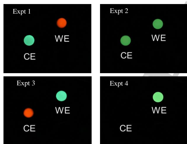
Figure 3. Photographs of the light emitted from the working electrode (WE) and counter electrode (CE) during the four experiments depicted in Fig. 2. Conditions: camera ISO 8000, aperture (f-number) 4 (Expt 1 and 2), 3.5 (Expt 3), and 11 (Expt 4).
