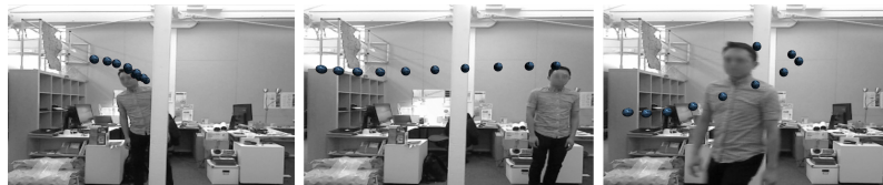
Figure 6. Ten digitally simulated SMRs forming a linear spline formation interact with the user's head movement. .
