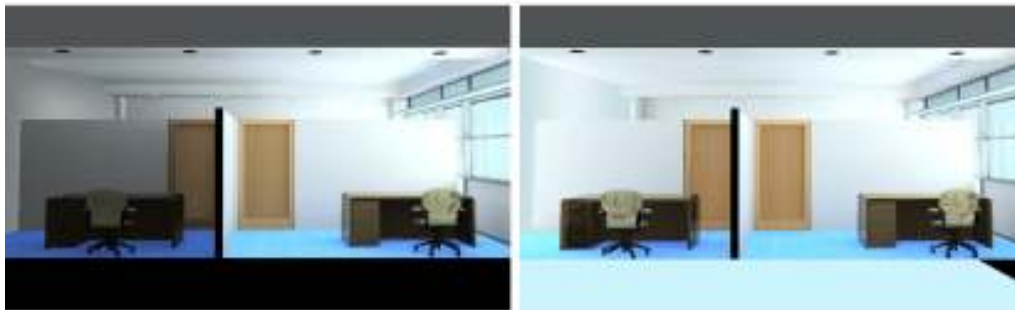
Figure 10 Room without clerestory light guiding blind (left) and with guiding blind (right).
