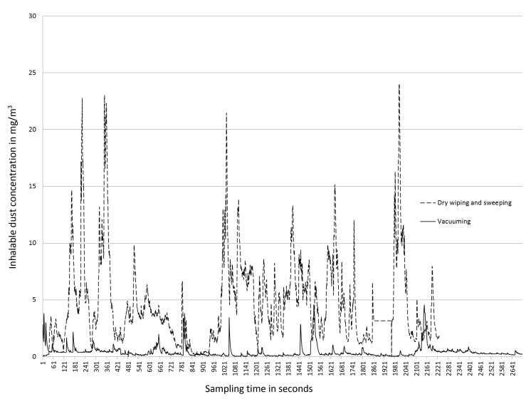
Figure 2. Inhalable dust concentrations (mg/m³) measured when dry wiping and sweeping (dashed line) versus dust concentrations measured when using a vacuum cleaner (solid line)
