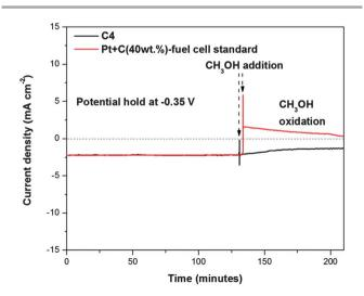
**Fig. 10** Chronoamperometric responses of  $C_4$  and Pt/C at -0.35 V in  $O_2$  saturated 0.1 M KOH without and with methanol at a rotating rate of 1600 rpm.
