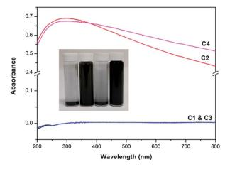
**Fig. 5** UV-Vis absorption of four samples after ultrasonic treatment.  $C_1$  and  $C_3$  quickly precipitate after ultrasonic treatment and indicate no UV-Vis absorption (inset:  $C_1$ – $C_4$  from left to right taken after 30 min of ultrasonication).
