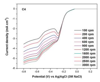
**Fig. 8** Rotating disk electrode (RDE) linear sweep voltammograms of  $C_4$  in  $O_2$  saturated 0.1 M KOH with different rotation rates at a scan rate of 20 mV s<sup>-1</sup>.
