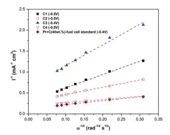
**Fig. 9** Koutechy–Levich plots derived from RDE voltammograms (at 1600 rpm) of different materials.
