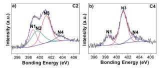
**Fig. 3** High resolution N1s XPS of (a)  $C_2$  and (b)  $C_4$ . The signal of  $C_2$  can be fitted with 4 components at 398.8, 399.7, 401.1, 403.6 eV, which correspond to pyridinic N (N<sub>1</sub>), pyrrolic N (N<sub>2</sub>), graphitic N (N<sub>3</sub>), and nitric oxide (N<sub>4</sub>). After annealing, pyrrolic N (N<sub>2</sub>) disappears and nitric oxide (N<sub>4</sub>) peak shifts to 403.1 eV.
