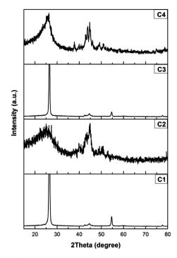
Fig. 2 XRD diffraction patterns of graphite after different treatments.
