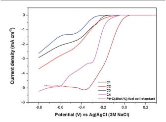
**Fig. 6** Rotating disk electrode (RDE) voltammograms of  $C_1$ – $C_4$  and Pt/C reference at 1600 rpm in  $O_2$  saturated 0.1 M KOH at a scan rate of 20 mV s<sup>-1</sup>.
