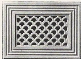
No. 1695 —Stamped Zinc Open Ventilator. Size: 9in. x 6in. For internal walls.
