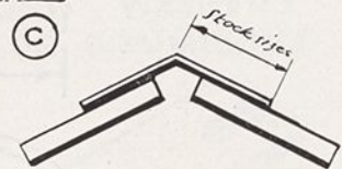
SECTION THRU RIDGE "C"
