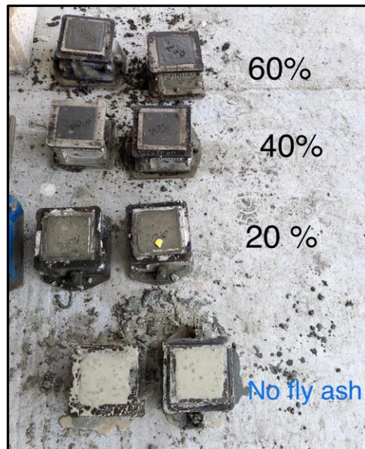
Figure 4. Image of the as prepared green concrete samples in the molds with different palm waste percentages.
