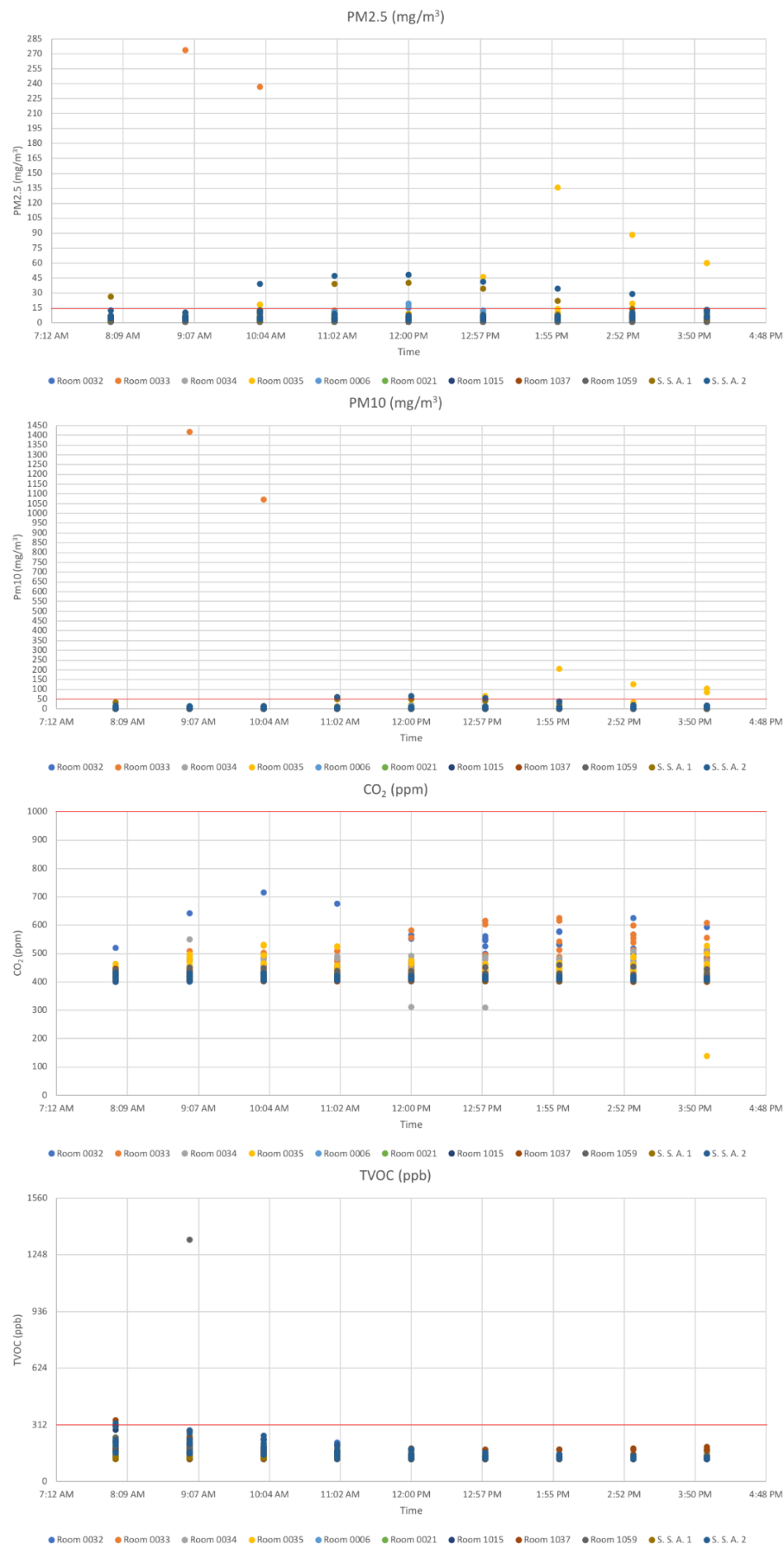
Figure 3. Hourly Based Indoor Air Quality Parameters (PM2.5, PM10, CO 2 , and TVOC).
