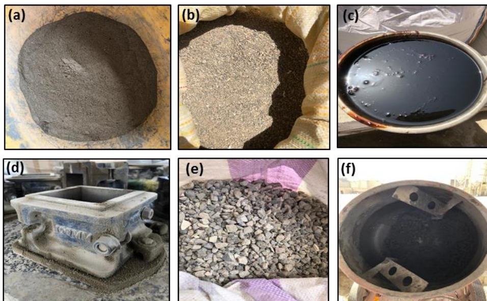
Figure 3. Components of ash powder; (a) Palm waste ash (b) Soft Aggregate (c) SP495X Sodamco/Fosroc (d) Mold 10 cm x 10 cm x 10 cm (e) Large aggregate (f) Mixer
