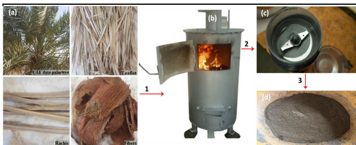
Figure 1. Preparing the palm waste ash steps; (a) the different components of lignocellulose wastes of UAE date palm tree, (b) Oven, (c) Grinder, (d) the obtained powder (palm ash).
