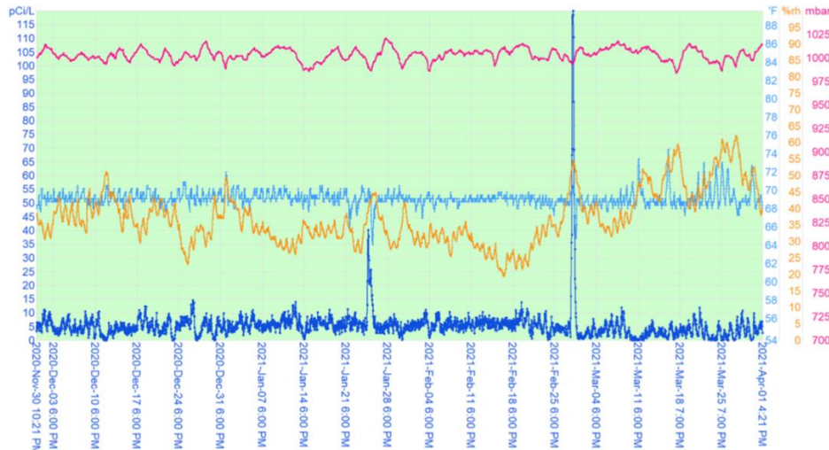
Figure 1. Indoor radon readings pCi/L aligned with indoor air temperature, relative humidity, and atmospheric pressure in house #1.
