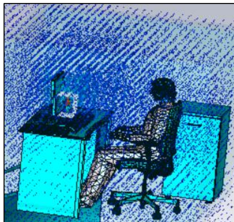
Figure 5. Electric field distribution for concrete at 2.45 GHz
