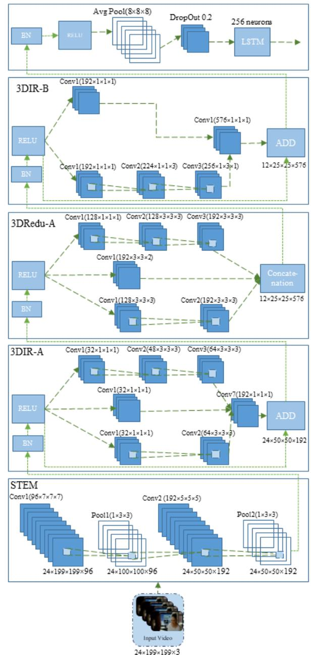
**FIGURE 2.** The 3D Inception-ResNet (3DIR)-LSTM architecture. (BN block shows a batch normalization node). The LSTM block containing 256 neurons is shown at the final stage of the structure, after extracting the spatial-temporal features from Inception-ResNet modules. The LSTM block output is fed to the classifier in the next phase.
