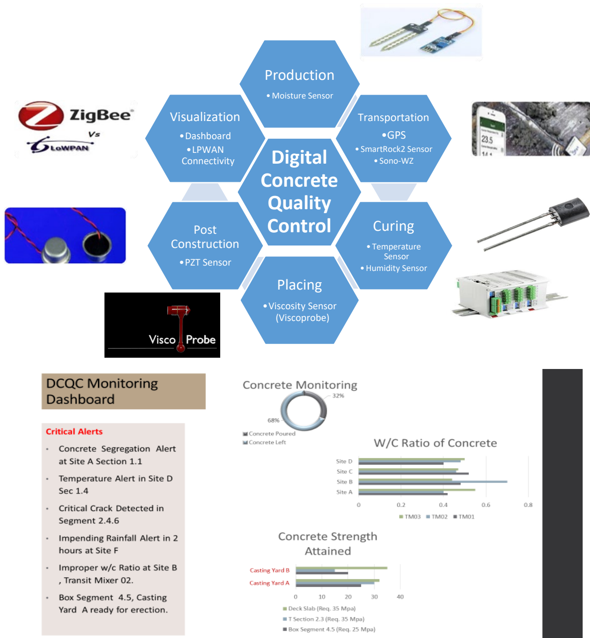
Fig.2 Proposed Framework and Dashboard for Digital Concrete Quality Control (DCQC) Monitoring
