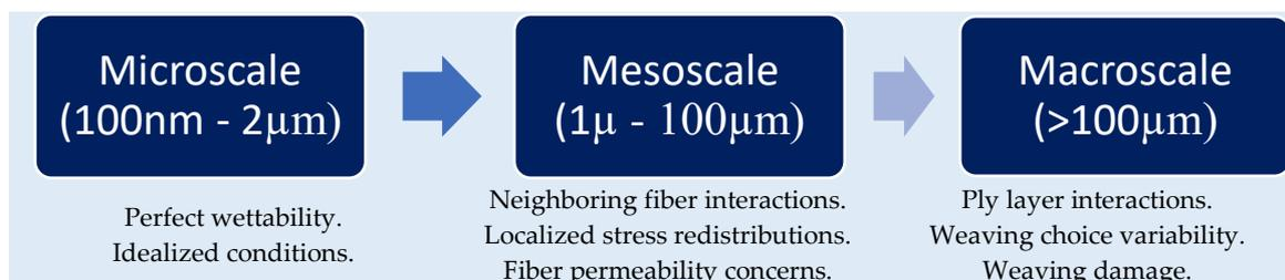
**Figure 1.** Graphic representing the different scales of testing and introduced testing variabilities.
