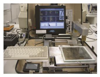
Fig. 1—OFDA instrument with liquid cell in measurement position (source: Textile Laboratory, Deakin University, Australia)
