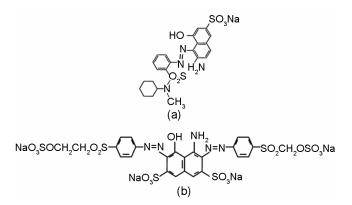
Fig. 2—Structures of (a) C I Acid Red 361, and (b) Lanasol Black CE<sup>68</sup>
