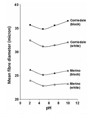
Fig. 3—Mean diameters of undyed and black dyed wool fibres in aqueous solutions at various pH
