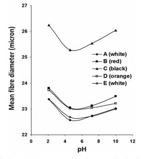
Fig. 4—Variation in dyed Merino fibre diameter as a function of pH
