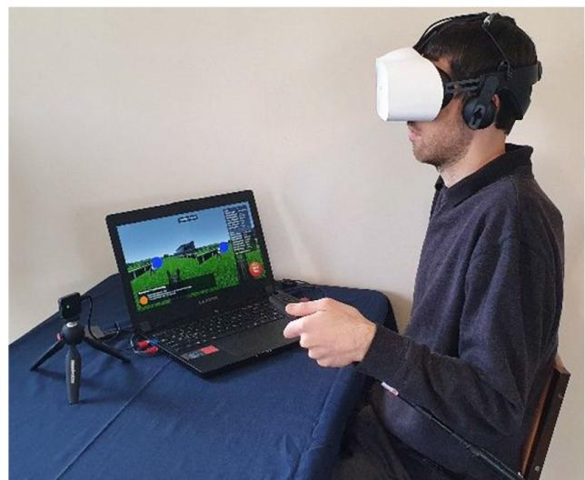
**Fig. 1** The CONVIRT test battery set-up, comprising the CONVIRT VR application, FOVE 0 Eye-Tracking VR Head-Mounted Display, riding crop with push button, running through a Gigabyte P35 laptop
