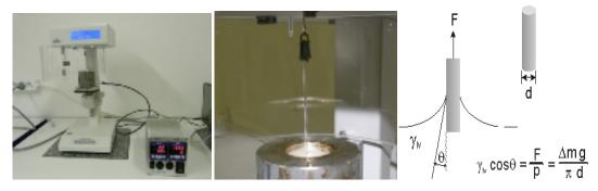
Figure 2. Measuring method for characterization of the surface tension of polymer melts.
