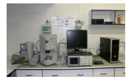
Figure 3. Rotation/vibration rheometer for characterization of flow properties of polymer melts.
